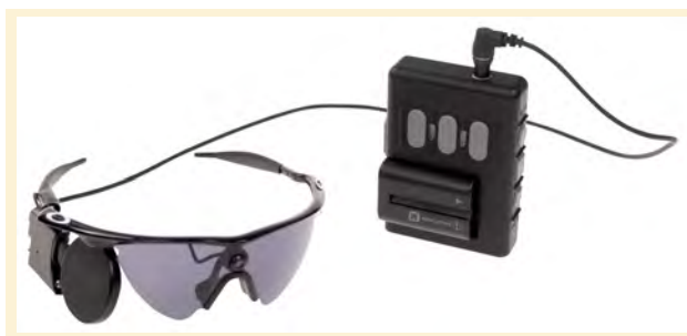
Figure 2. The external equipment includes glasses, a camera, a video processing unit (VPU) and a cable.
